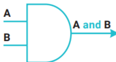
2-rasm. "AND" elementi
